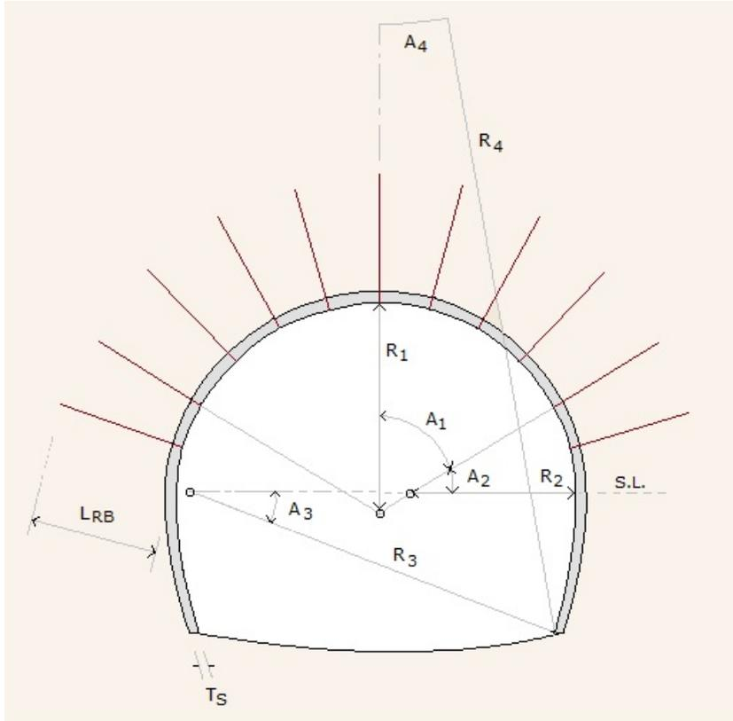
Figure 4.2a Horseshoe shape tunnel dimension
