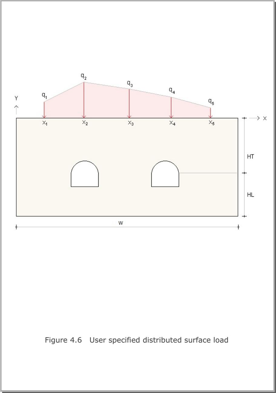
Figure 4.6 User specified distributed surface load
