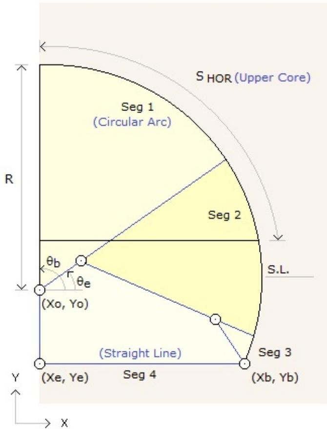
Figure 4.2c User defined tunnel dimension for ISTYPE = 3
