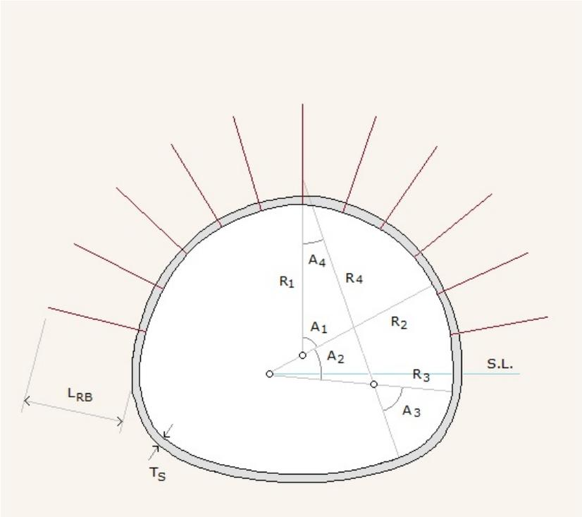
Figure 4.2b Egg shape tunnel dimension
