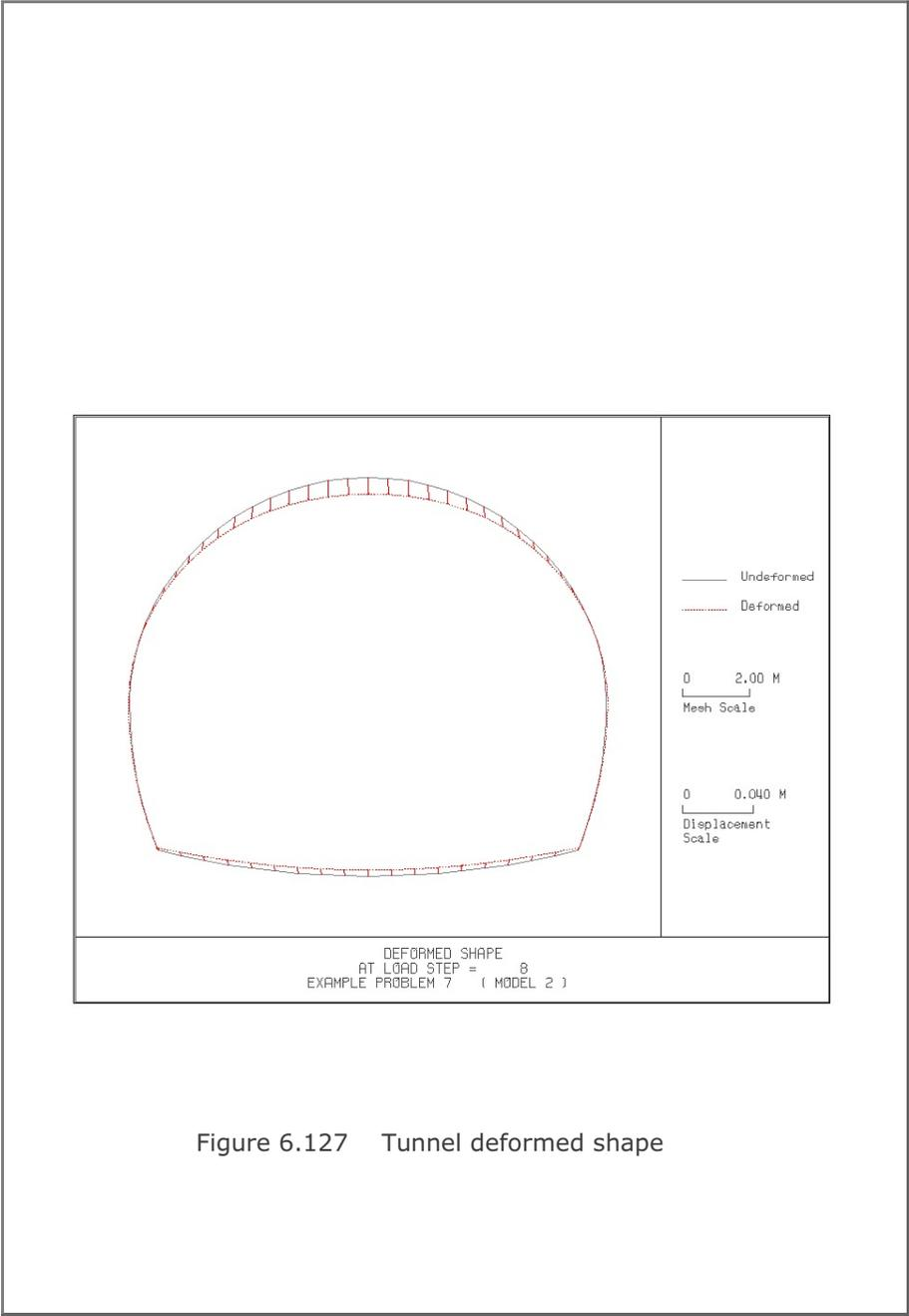
Figure 6.127 Tunnel deformed shape
