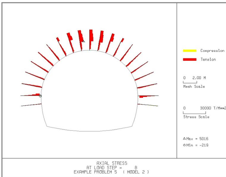
Figure 6.115 Rock bolt axial stresses
