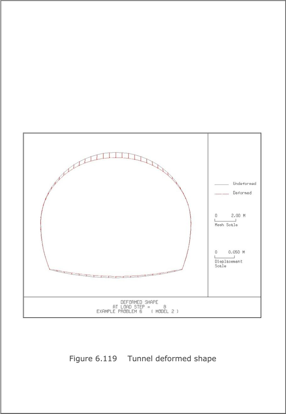
Figure 6.119 Tunnel deformed shape
