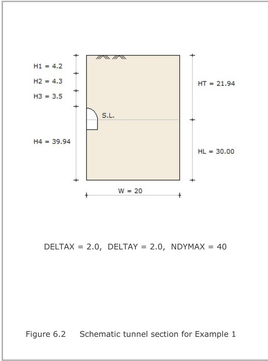
Figure 6.2 Schematic tunnel section for Example 1
