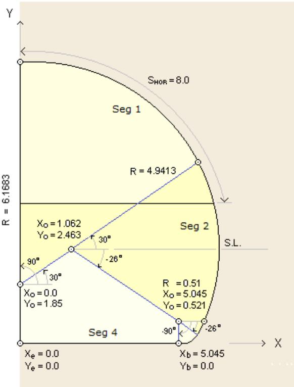
Figure 6.132 Dimensions of right tunnel for Example 8
