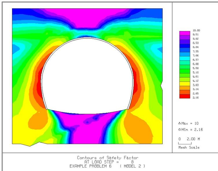
Figure 6.122 Contour of safety factor
