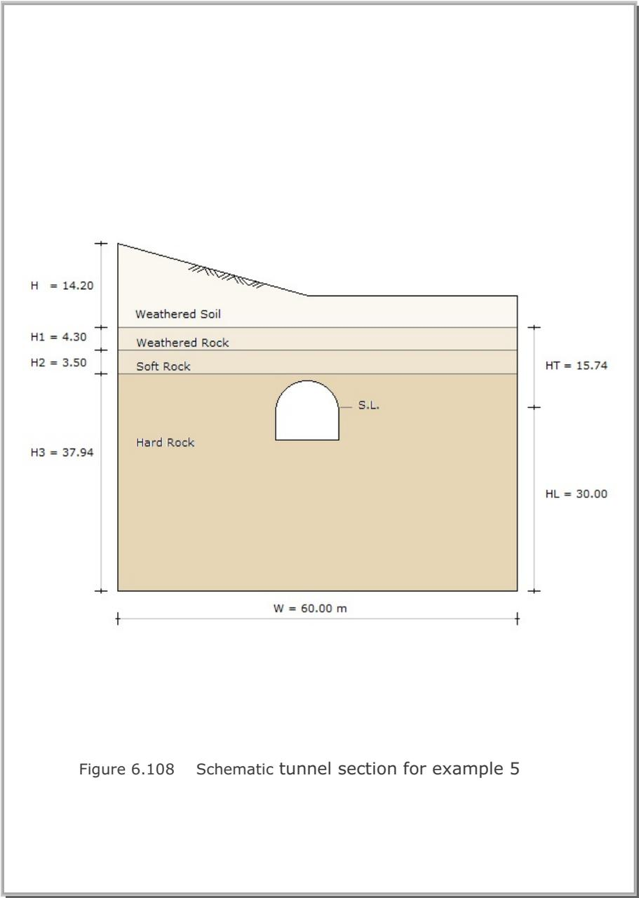
Figure 6.108 Schematic tunnel section for example 5
