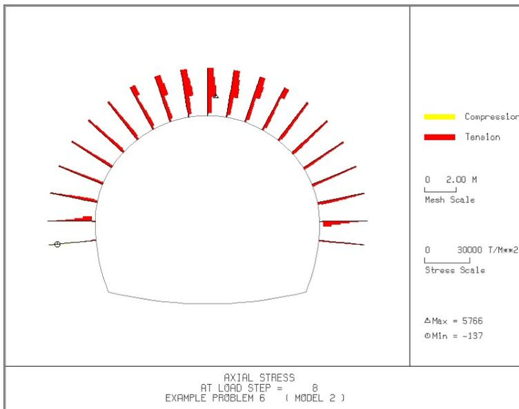
Figure 6.123 Rock bolt axial stresses
