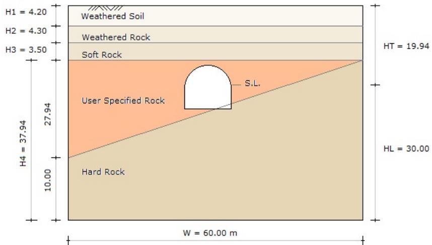
Figure 6.116 Schematic tunnel section for Example 6
