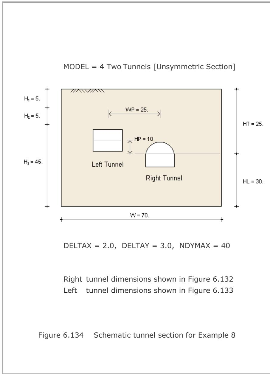
Figure 6.134 Schematic tunnel section for Example 8
