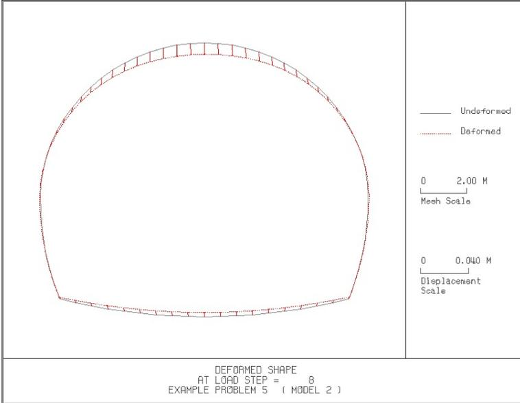
Figure 6.111 Tunnel deformed shape
