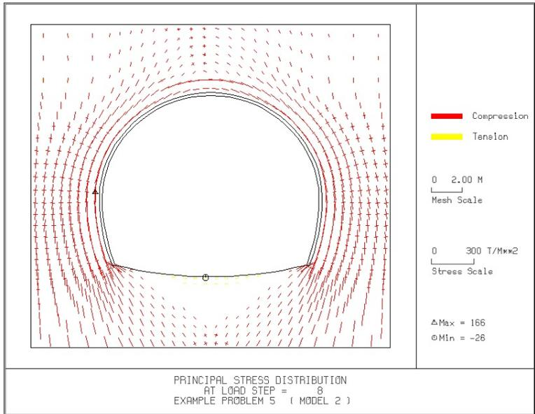
Figure 6.112 Principal stresses around tunnel
