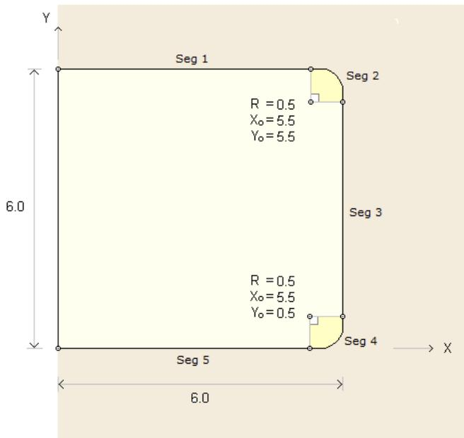
Figure 6.133 Dimensions of left tunnel for example 8
