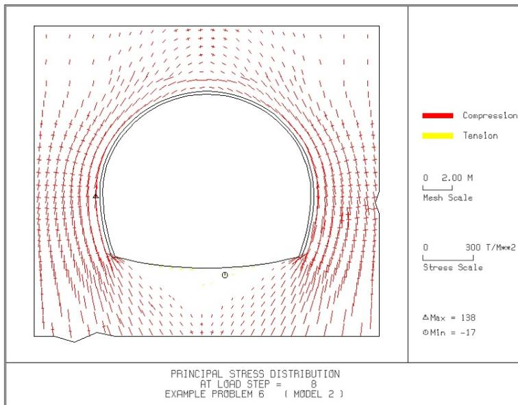
Figure 6.120 Principal stresses around tunnel
