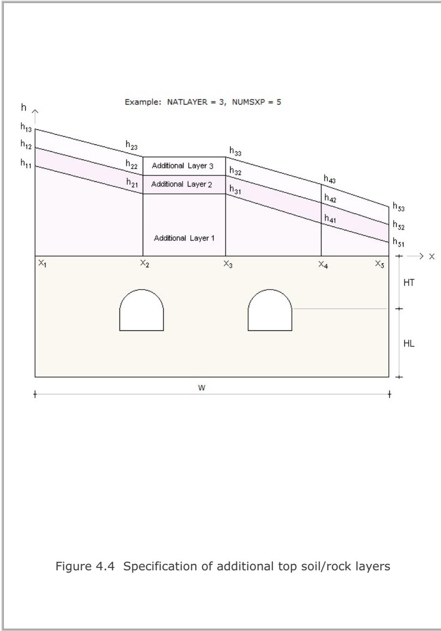
Figure 4.4 Specification of additional top soil/rock layers
