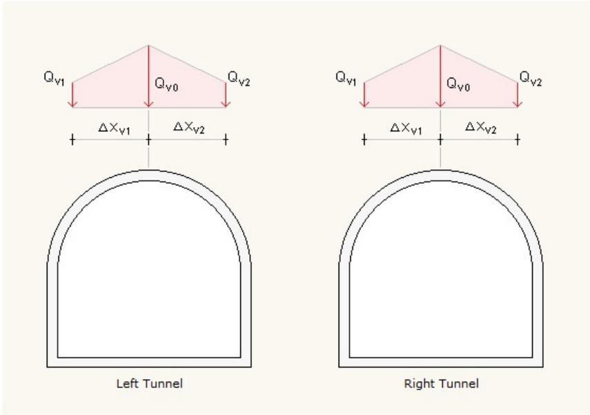
Figure 4.7 Additional vertical loosening load
