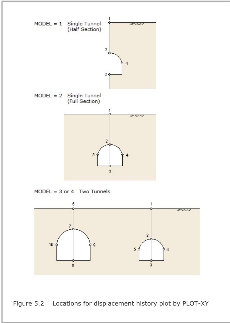
Figure 5.2 Locations for displacement history plot by PLOT-XY
