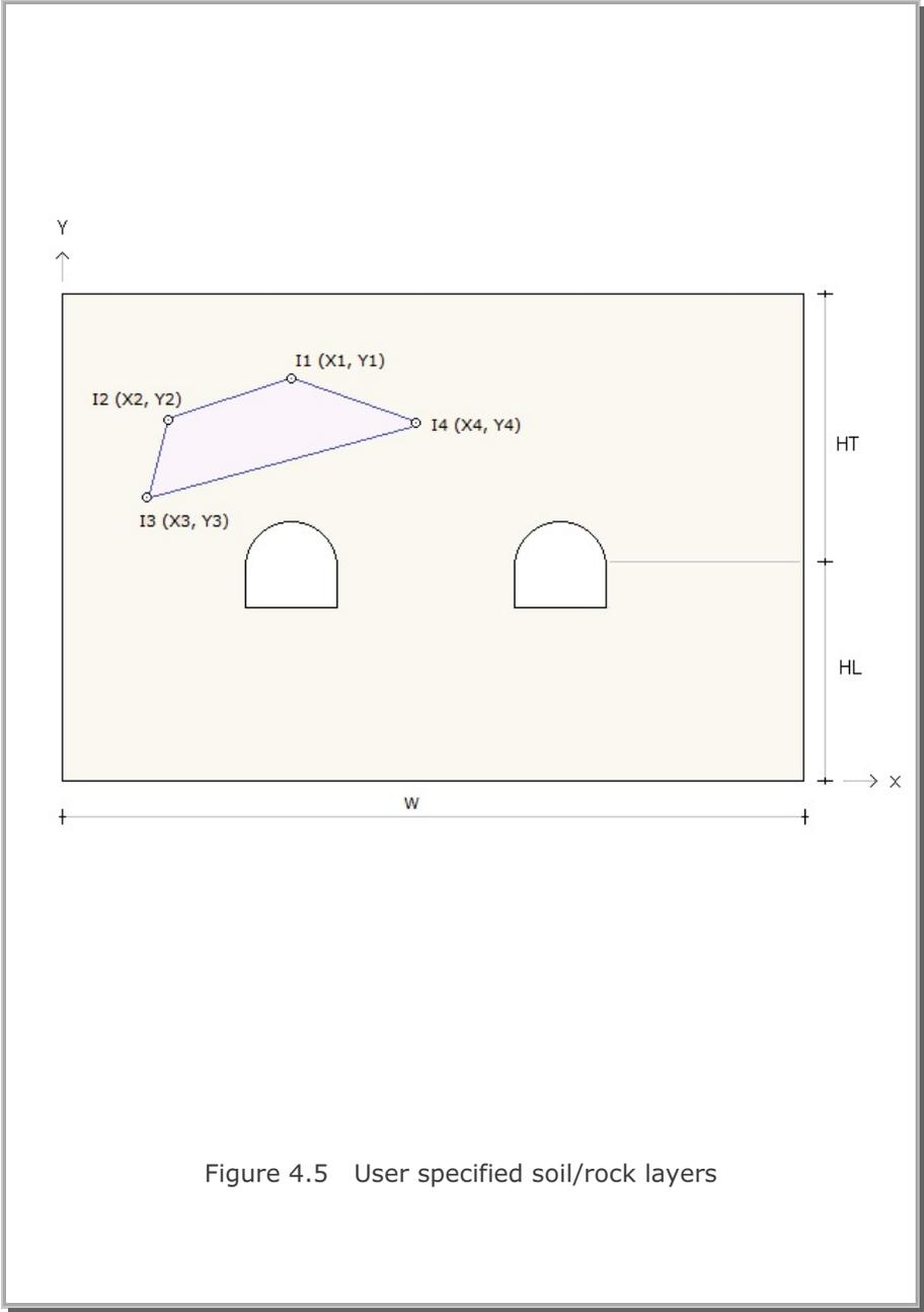
Figure 4.5 User specified soil/rock layers
