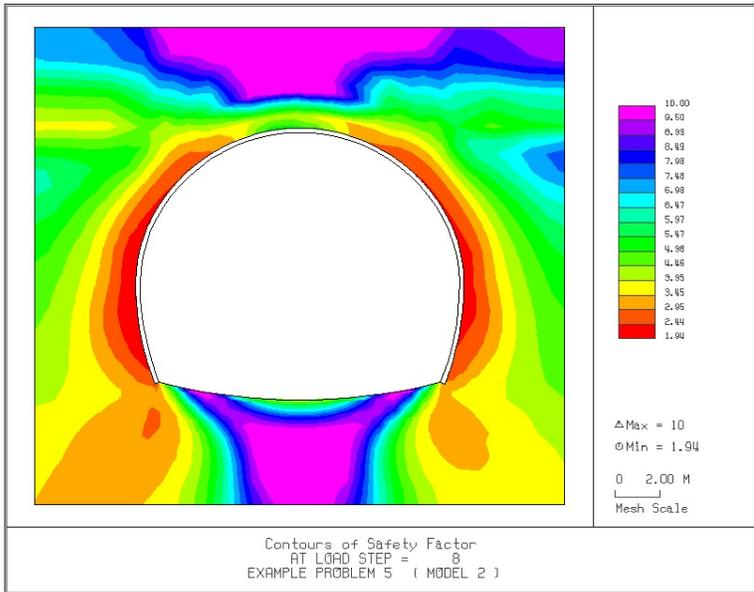
Figure 6.114 Contour of safety factor
