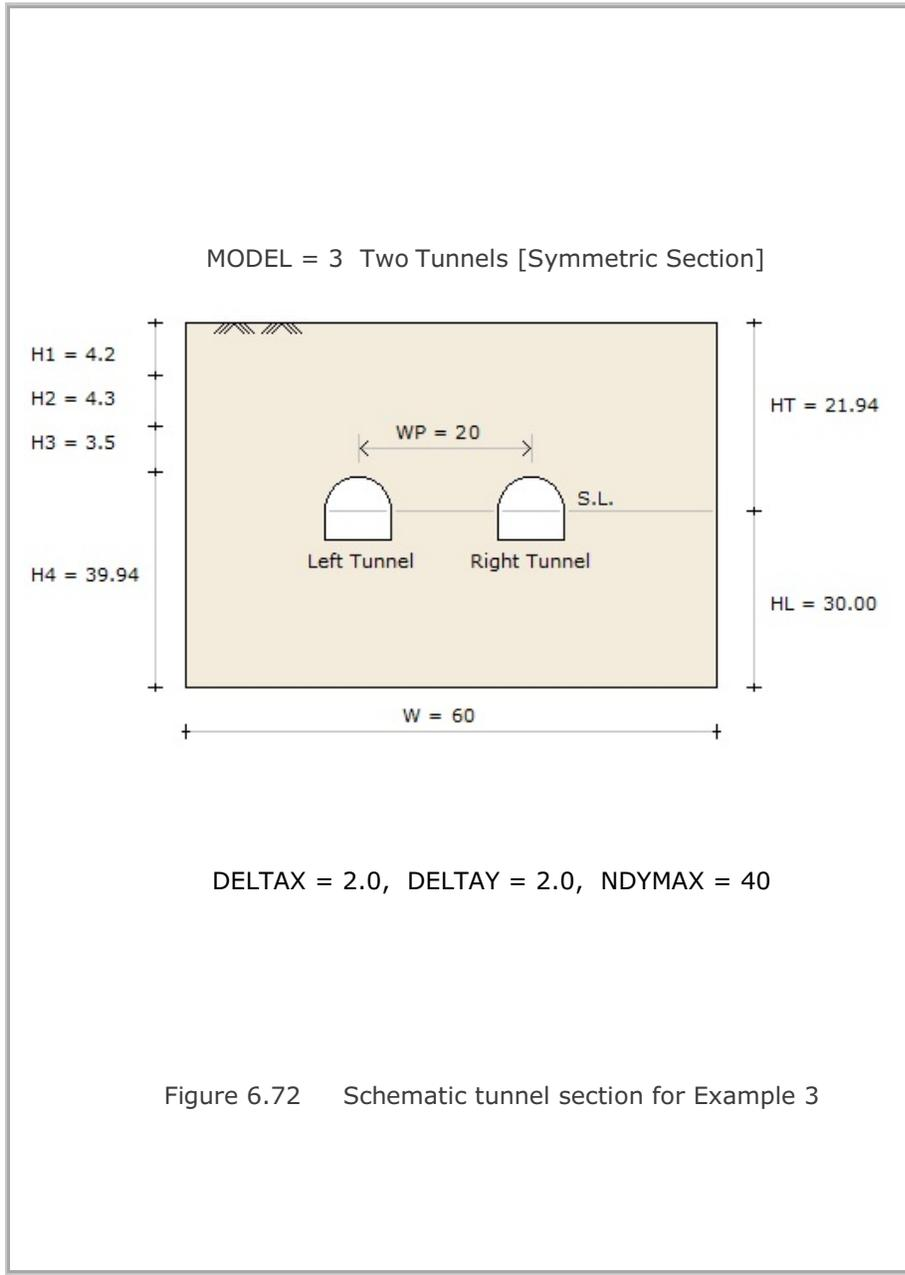
Figure 6.72 Schematic tunnel section for Example 3
