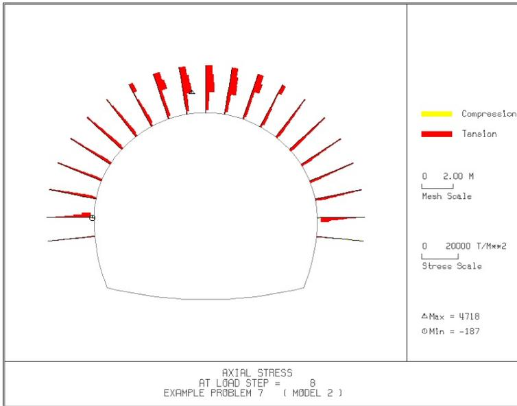
Figure 6.131 Rock bolt axial stresses
