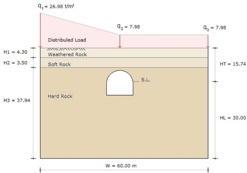
Figure 6.124 Schematic tunnel section for example 7
