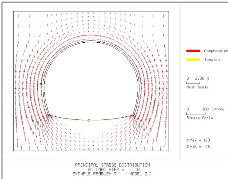
Figure 6.128 Principal stresses around tunnel
