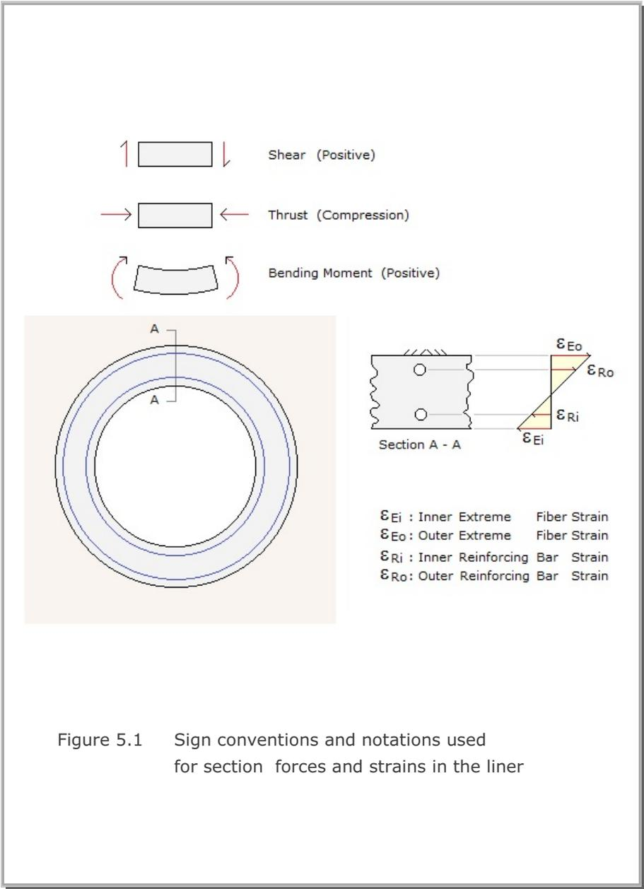
Figure 5.1 Sign conventions and notations used for section forces and strains in the liner
